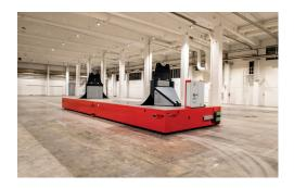
Solving provides a wide range of automated handling systems for customers in the paper industry: AGVs, air film Movers, wheeled and railed handling equipment. The handling systems can be used not only for the handling of tambour rolls but also for handling paper reels, cores and sheet pallets.
