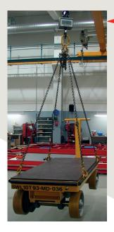
Lifting eye bolts allow the trolley to be lifted by crane.
