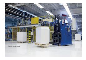
Solving provides a wide range of automated handling systems for customers in the paper industry: AGVs, air film Movers, wheeled and railed handling equipment. The handling systems can be used not only for the handling of sheet pallets but also for handling paper reels, tambour rolls and cores.
