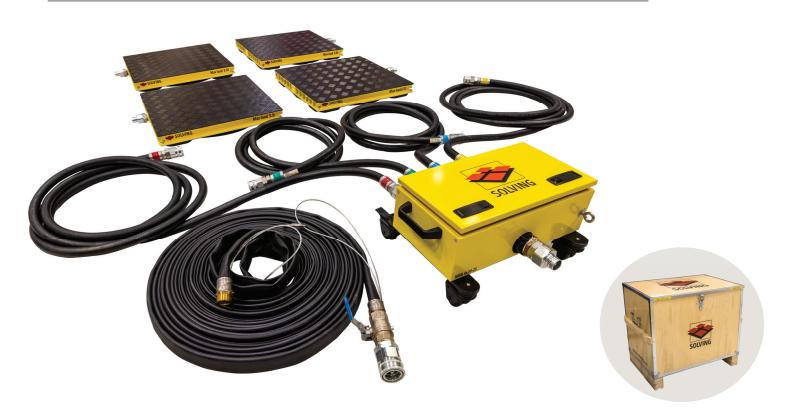
Solving MLS Modular Air Bearing Systems are designed to move any load, large or small, from a few thousand kilos to 360 tons.
