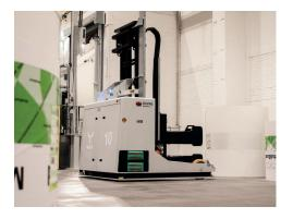
Solving provides a wide range of automated handling systems for customers in the paper industry: AGVs, air film Movers, wheeled and railed handling equipment. The handling systems can be used not only for the handling of paper rolls but also for handling of sheet pallets, tambour rolls and cores.
