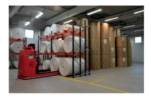
Solving provides a wide range of automated handling systems for customers in the paper industry: AGVs, air film Movers, wheeled and railed handling equipment. The handling systems can be used not only for the handling of paper reels but also for handling of sheet pallets, tambour rolls and cores.
